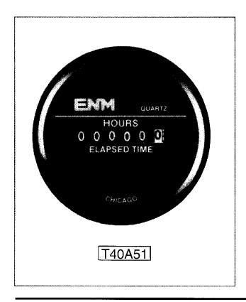
ENM's new hour meter operates only when the engine is running. This unique feature is accomplished by sensing the output from the engine's alternator. When the engine is operating, the system voltage increases above the battery voltage. This increase is detected and the hour meter starts accumulating time.
